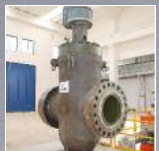
Through Conduit Expanding Gate
