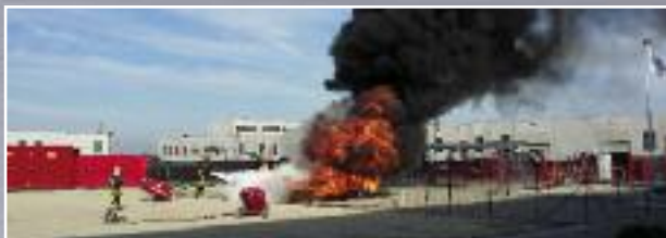
Fire test with twin-agent foam powder wheeled unit ta 100-100
